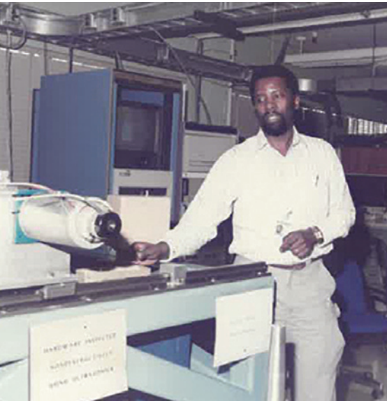
MATERIALS TEST — In the early 1980s, Marvin Kelley showed off the Automatic Multi-axis Ultrasonic Scanner, or AMUS, that he helped design and build to test materials at Sandia.
