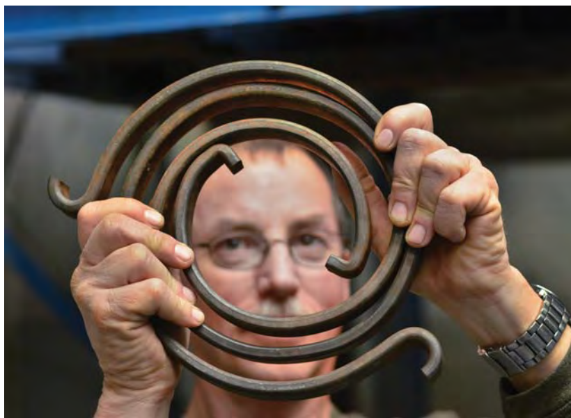
Elton Wright (6916) shows a torsional spring that's used to simulate the rotational vibration of the drill string in a Sandia experiment. (Photo by Randy Montoya)
