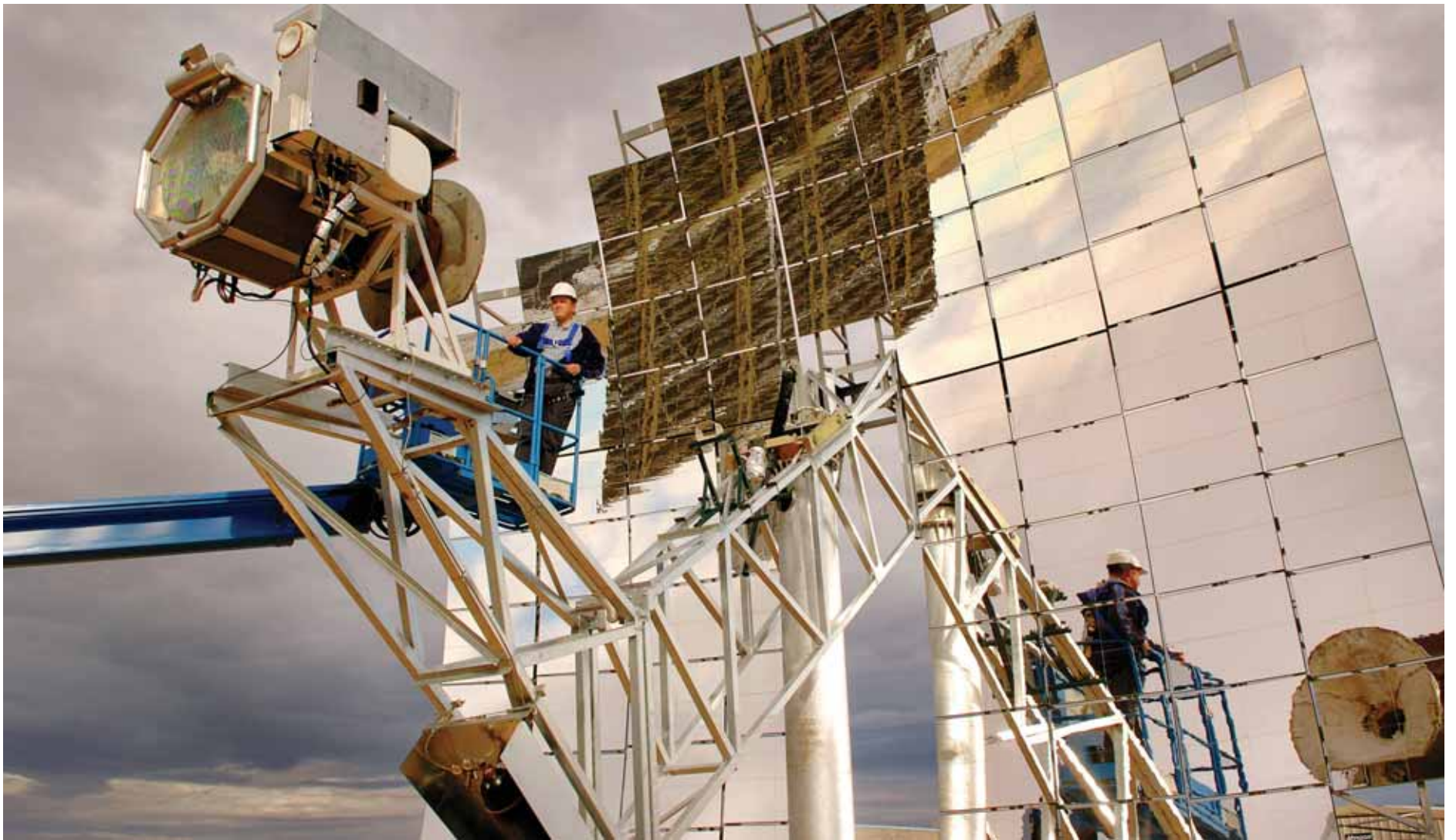
SANDIA RESEARCHER CHUCK ANDRAKA makes adjustments to a Stirling Energy Systems, Inc. solar dish-engine system installed at Sandia's National Solar Thermal Test Facility earlier this year. Five more will be erected by January as test units. (Photo by Randy Montoya)
