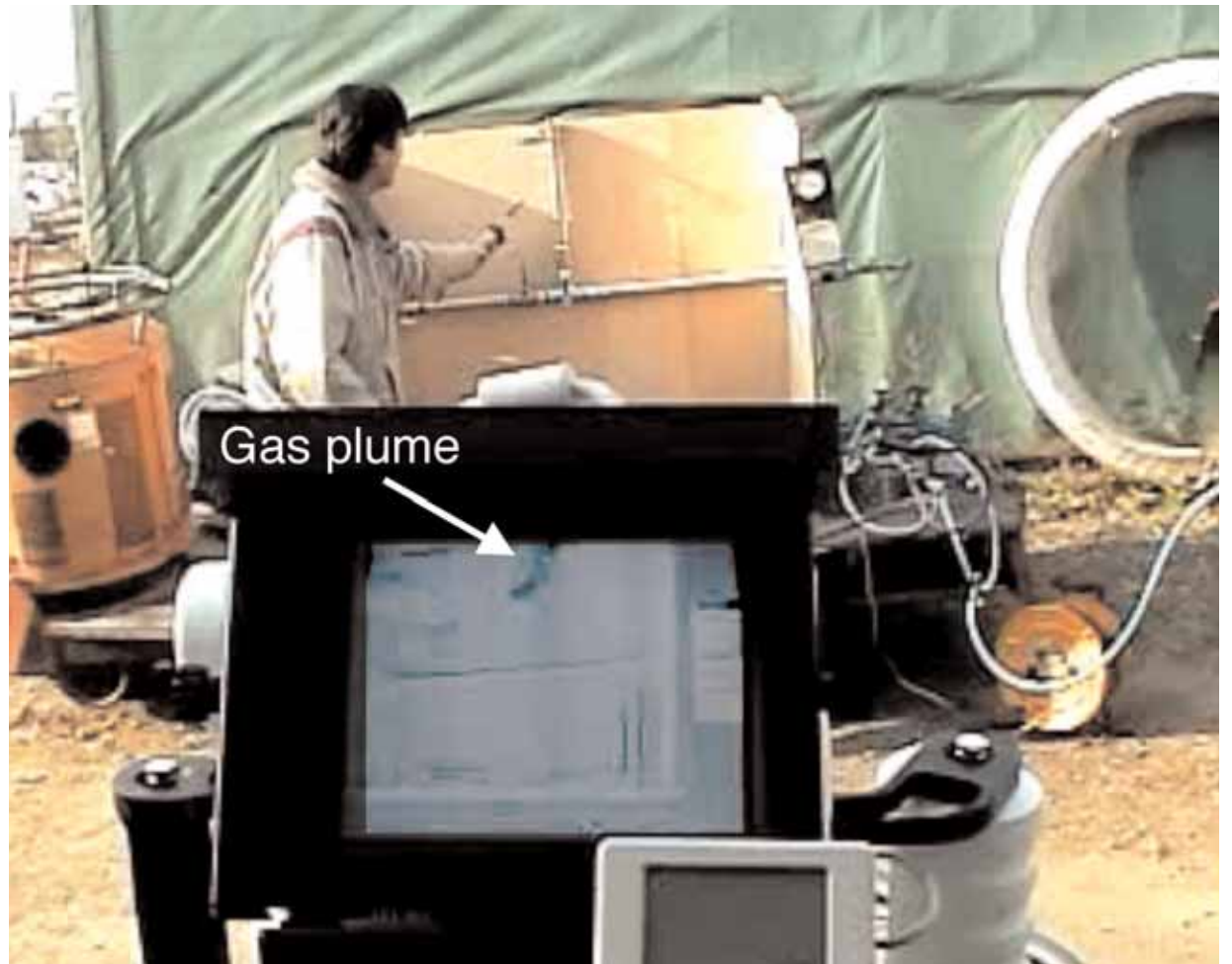
VIEW OF THE GAS IMAGE on the portable gas imager monitor when operating in differential imaging mode. The person in background is measuring the plume with a handheld sensor.
