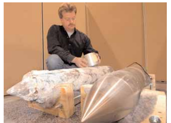
MARK PILCHER takes a look at a TACMS-P after test (left) and a mass mockup (right) used for system testing.
