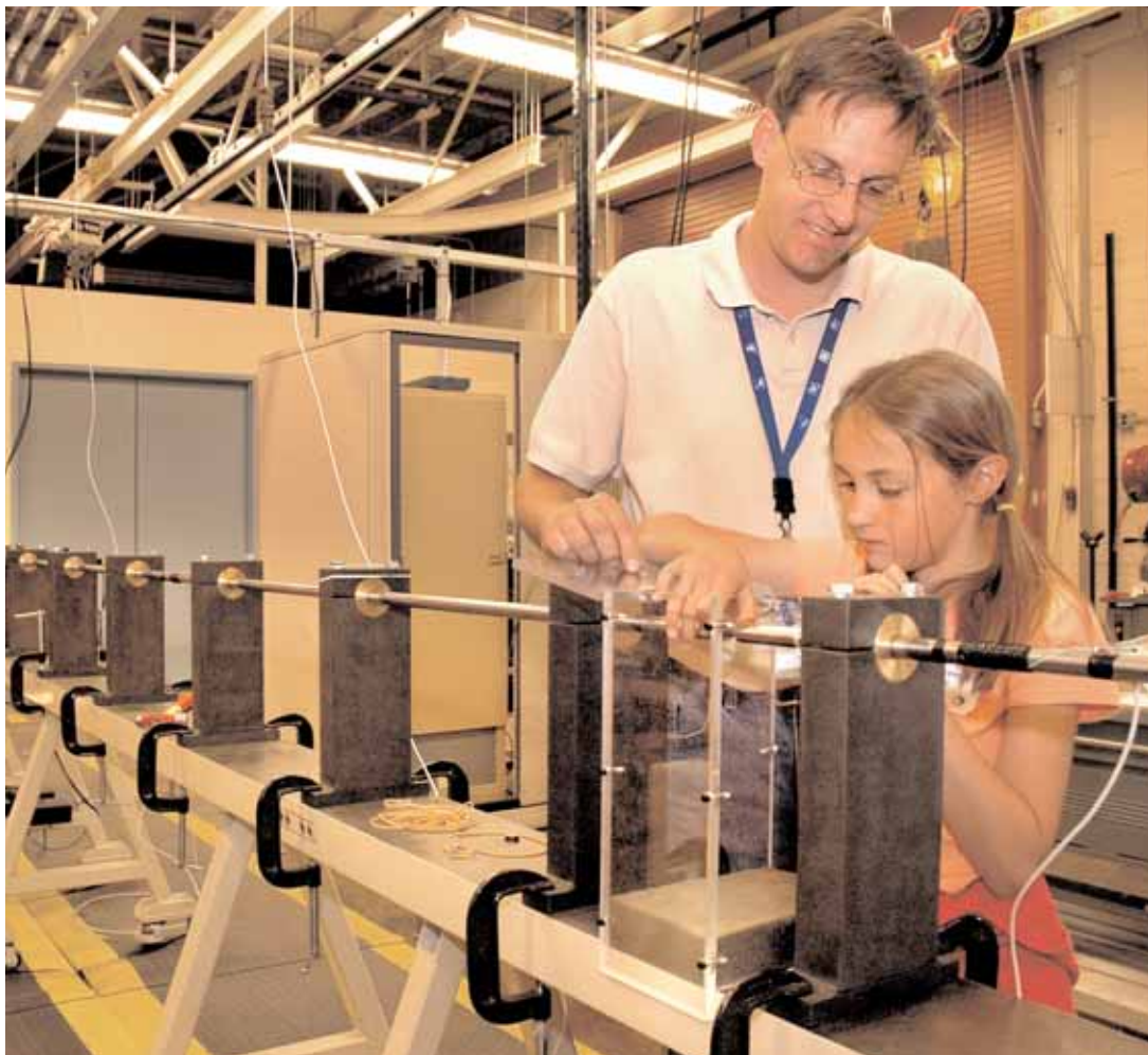
GOOD VIBRATIONS — Blythe Frew and her dad Danny (15412) set up a sample for a shock test in a Hopkinson Bar Lab. (Photo by Amanda Montoya, age 10)
