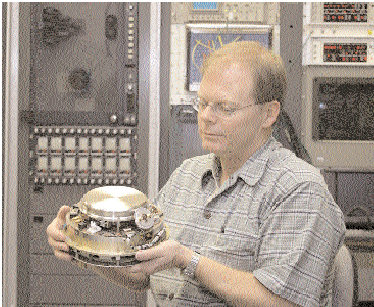
COMPACT — Rex Eastin examines the substantially reduced telemetry subassembly of the W76-1 joint test assembly, JTA1. It is less than two-thirds the size of its predecessor. (Photo by Bud Pelletier)
