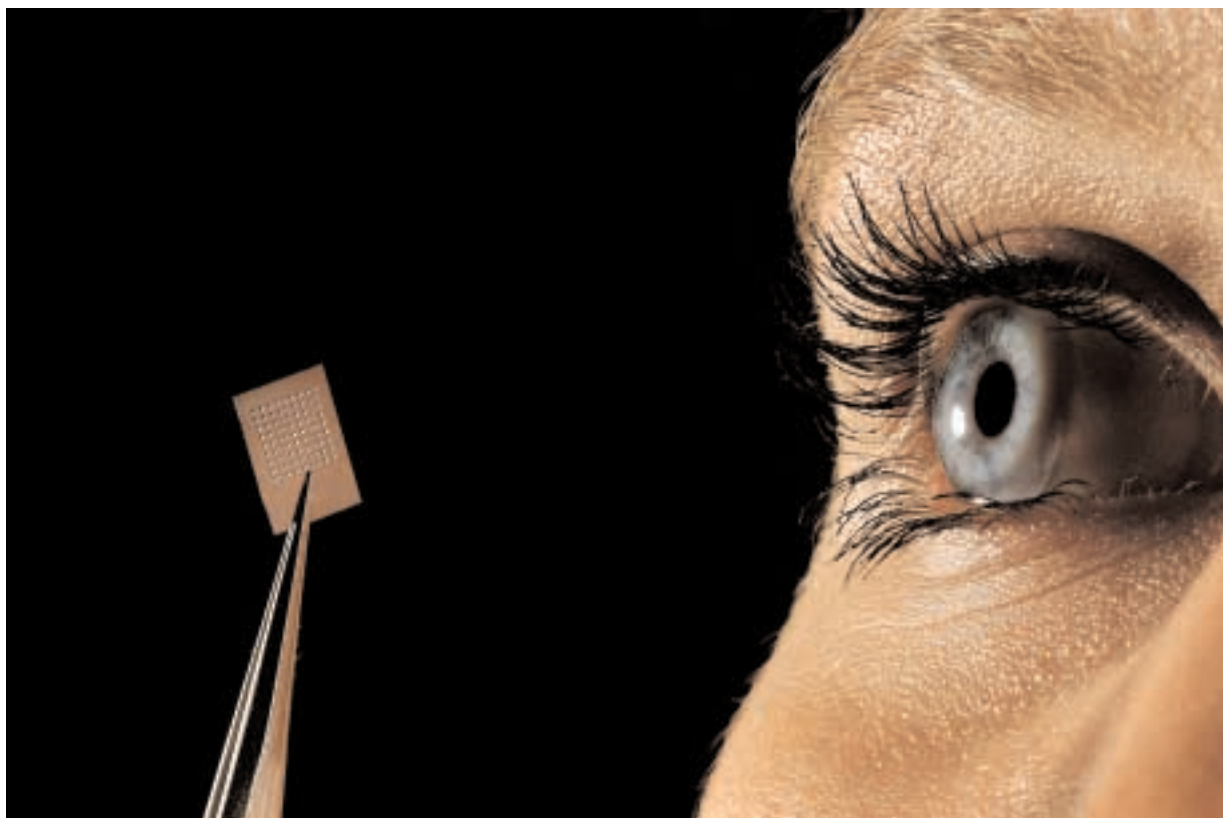
THE EYES HAVE IT — A prototype of the MEMS-based array that eventually may be inserted into the retina of a blind patient. The design is by Murat Okandan (1749). (Photo by Randy Montoya)
