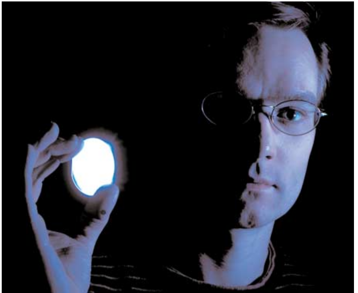
NEW WHITE LIGHT — Art Fischer (1123) holds a sapphire substrate with indium gallium nitride layers. This is the base material for one type of semiconductor light-emitting diodes (LEDs). (Photo by Randy Montoya)
