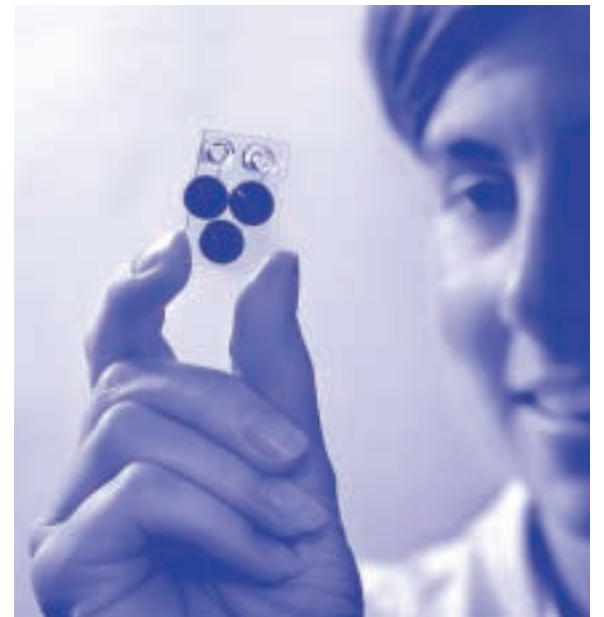
CHANNELING — Kate Smith, a former postdoctoral student in the microChemLab group, holds a fused silica wafer bearing microchannels. (Photo by Randy Montoya)
