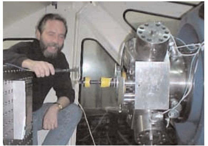
CHARACTERIZATION TESTS — Jim Lauffer (8727) strikes the end of a milling machine cutting tool with an instrumented hammer. One way Sandia characterized the structural dynamics of the machine was by exciting the cutting tool with a known input force and measuring its response using accelerometers mounted on the tool.
