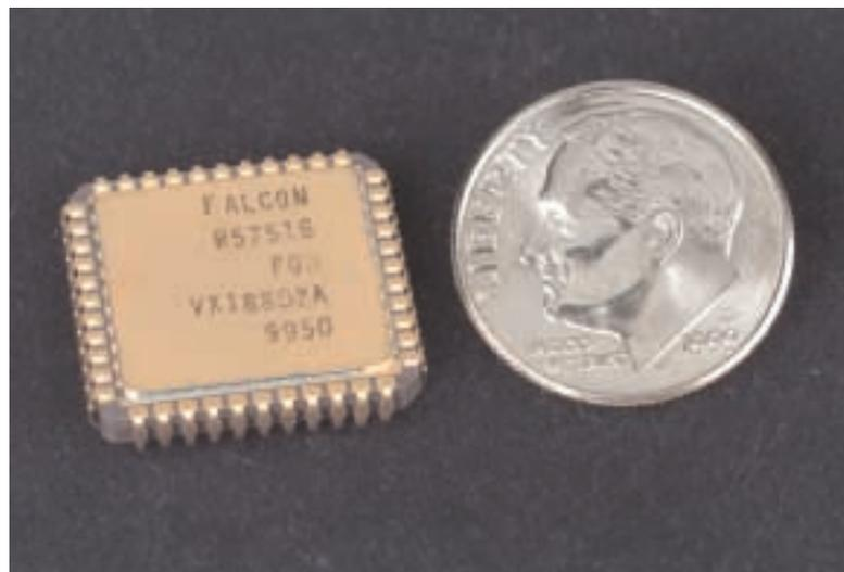
PULSE STRETCHER technique of Ken Condreva's FALCON integrated circuit, seen here larger-than-life-size next to a Roosevelt dime, makes it a high-resolution, low-cost timekeeper extraordinaire.
