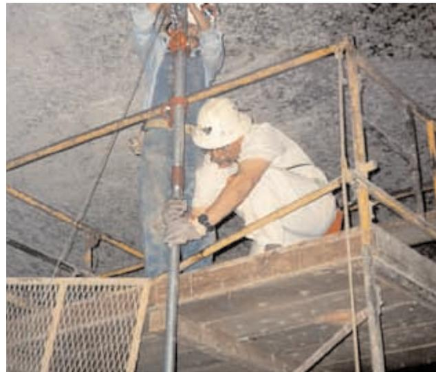
MINE CHECK — Sandian Steve Bauer (6113), on top of a scaffold in the Norton mine, runs a test to assess the mine's *in situ* permeability.
