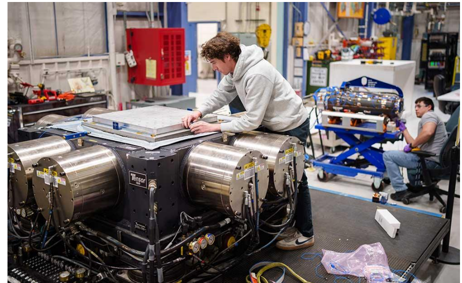
6-DOF Shaker Table for MIMO Testing [2]
