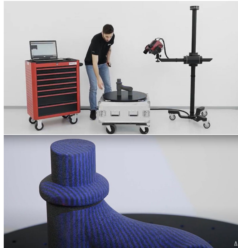
Fig. 7 ATOS Compact Scan – Blue Light 3D Scanner. https://www.youtube.com/watch?v=T-RkQioXHYg
