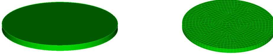
Figure 2-68. – PZT5A disc verification problem.
