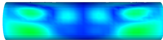
Figure 7-5. – Wet Modes Results. The mode shapes from wet modes can be visualized like any other Eigen solution case.
