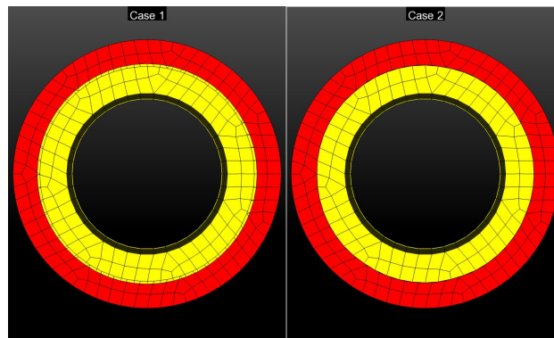
Figure 3-20. Small overlap and results after overlap removal
