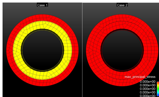
Figure 3-23. Stresses experienced after overlap removal
