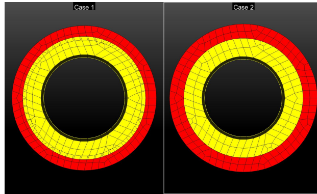
Figure 3-22. Large overlap and results after overlap removal method
