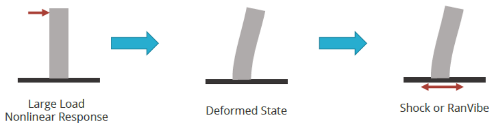
Figure 3-1. – Applying Sierra/SD to the output of Sierra/SM : cantilevered beam.
