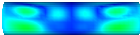
Figure 8-6. – Wet Modes Results. The mode shapes from wet modes can be visualized like any other Eigen solution case.
