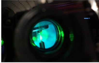
Fig 3-18. View looking back down the vacuum port through the imaging optics. The bright central part of the barbell is visible, together with the cathode at the top of the image.
