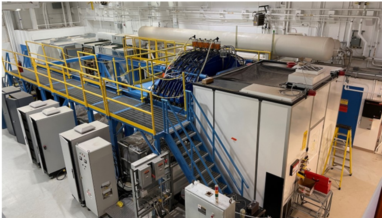
Figure 5.1. The SNL Mykonos facility [36]. On the left of the image is the machines charging power supplies, located in white electronic racks. The five vertically orientated disks are the machine's cavities, rendered for a better view in Fig. (5.2). The white room located in front of the five cavities is the Laser Controlled Area (LCA) and is where the vacuum chamber is located.
