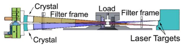
2 Z-Beamlet 2x x-ray laser beams crystals hit 2 targets Be liner at Z center camera snout 2× return apertures
