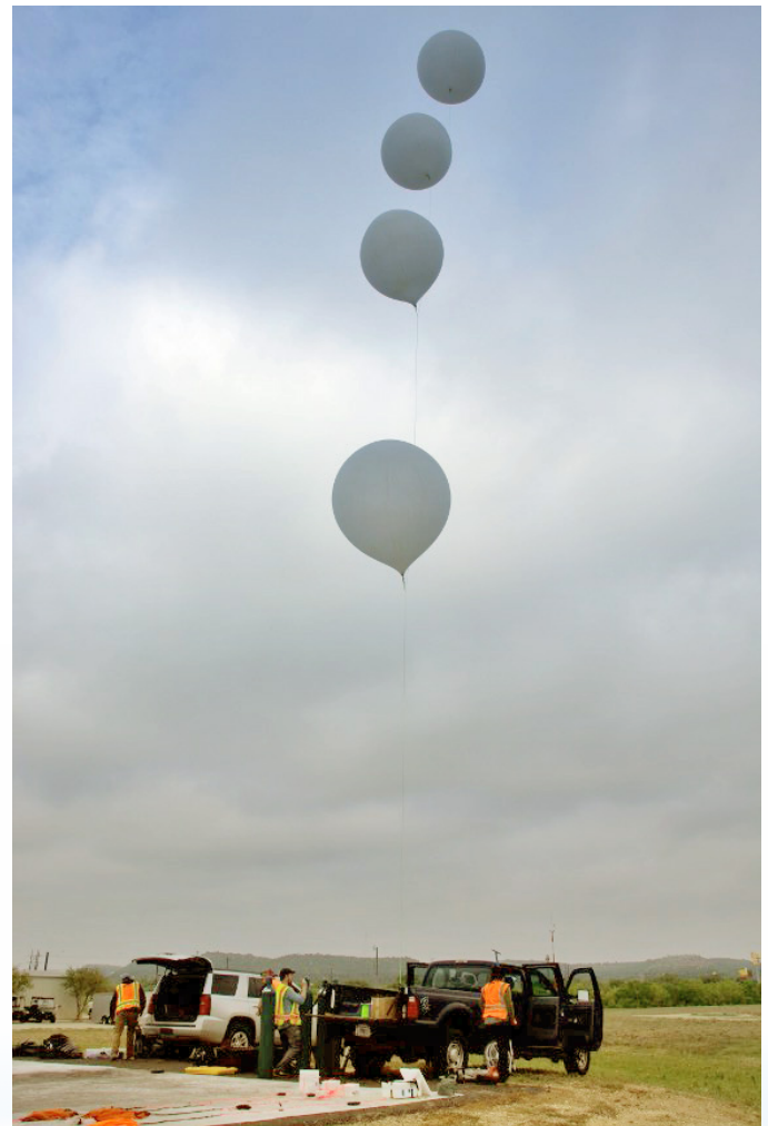
Four solar-powered heliotropes rigged for a weather-balloon assisted ‘grand slam’ launched from Texas by Sandia National Laboratories hours before totality of the Great American Eclipse on April 8, 2024.
