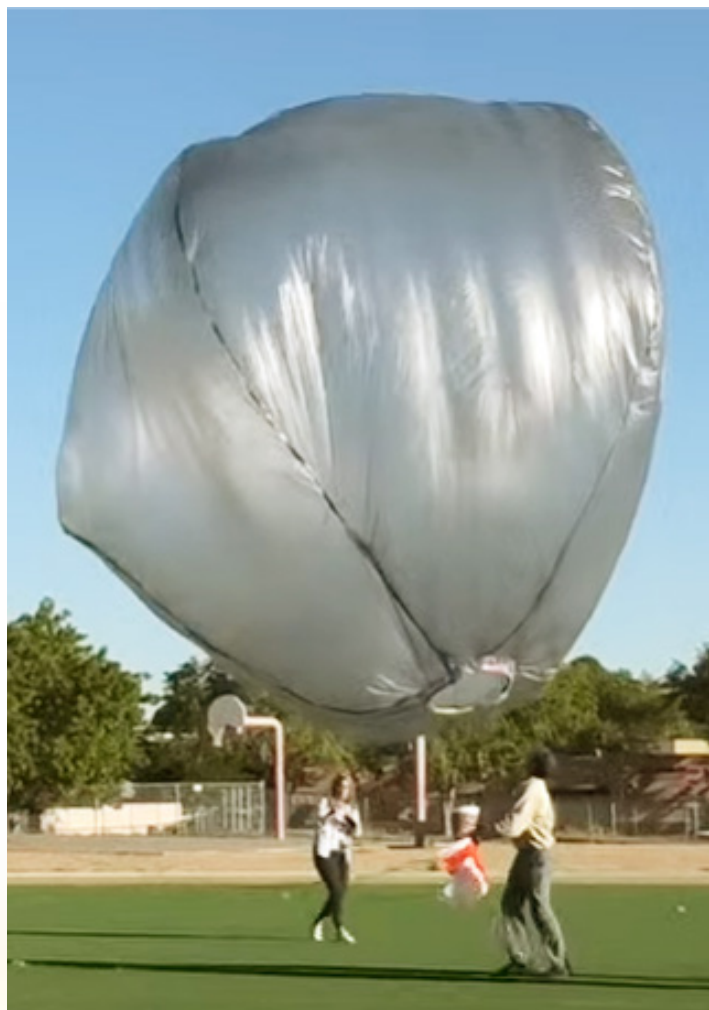
This heliotrope built by Cleveland Middle School students contained a seed-exposure experiment, flew for 13 hours, and landed 127 miles from its launch site.
