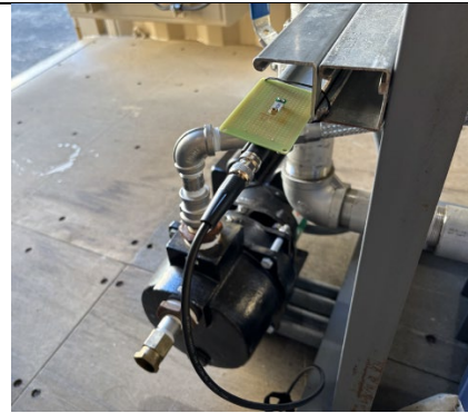
Figure 11. Vibration and Temperature Probe Details
