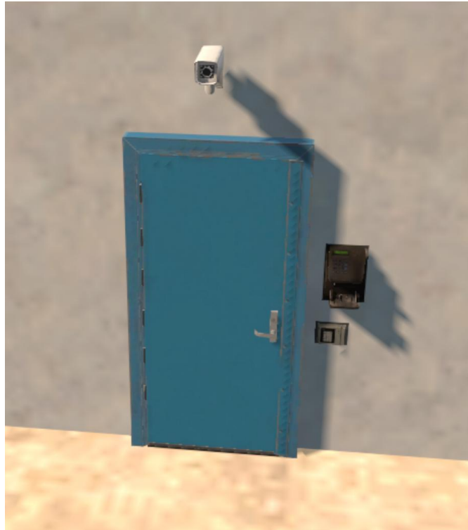
Figure 5. Exterior Door Physical Protection Measures
