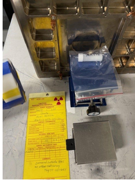
Figure 5. An example of when the sample is placed on a raised stage to align the sample with the SOFIA detector window. The HPGe snout is pictured to the left.
