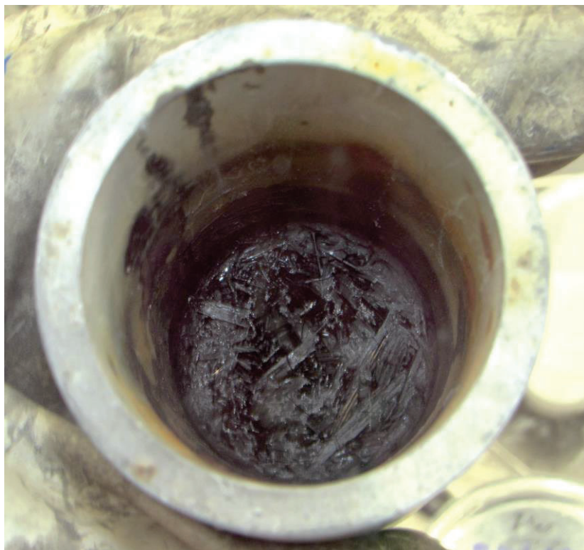
Figure 17. LiCl-KCl-UCl 3 (72.3 wt% UCl 3 ) solidified in a boron nitride crucible.
