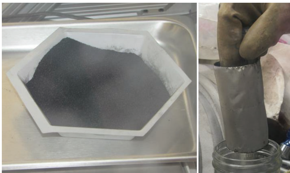
Figure 21. Natural uranium powder precursor (left) and stainless steel mesh basket (right).
