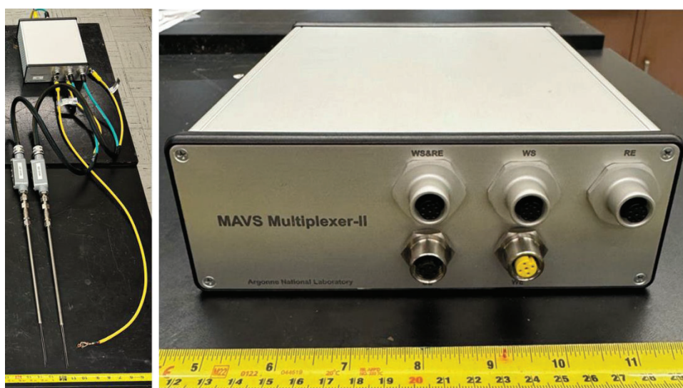
Figure 8. Picture of a multielectrode array voltammetry sensors (MAVS) and multiplexer system.
