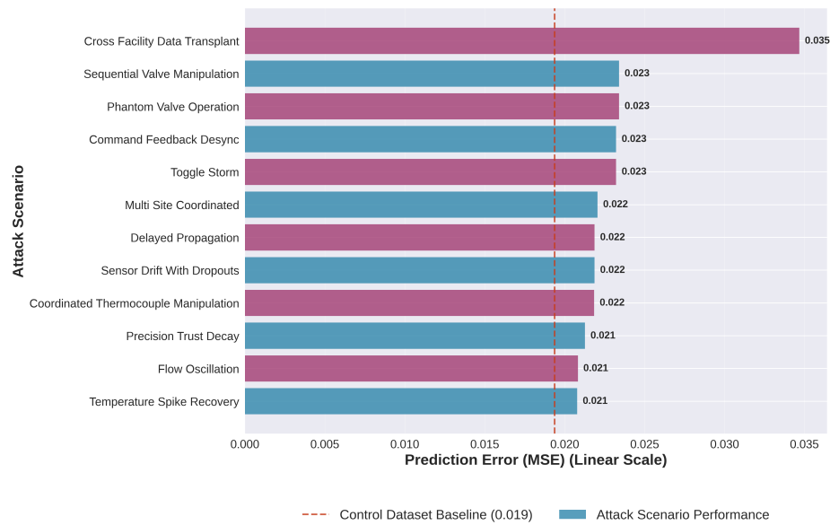
LSTM Anomaly Detection Performance by Attack Scenario Prediction Error (MSE) Analysis for Cybersecurity Detection with Control Baseline
