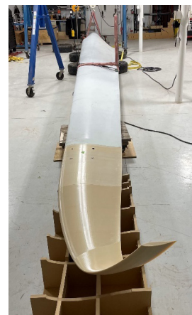
AMSIT tip and winglet mounted on a blade at SWiFT (Photo by Brent Houchens).
