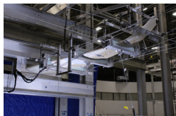
AMSIT test article with in-plane, centrifugal, and normal loads applied at 80% of design load (Photo by NIAR).
