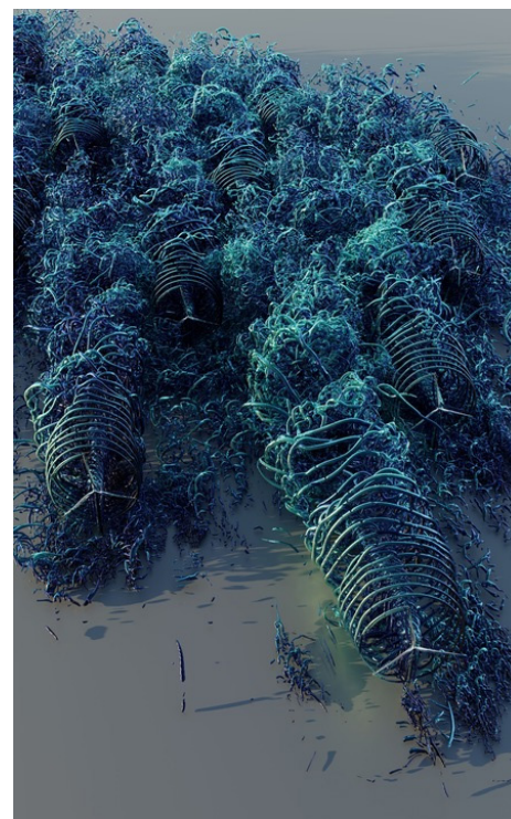
Illustration of the vortical structures in the downstream wakes of the geometry-resolved, 16 NREL 5MW turbine simulation (Graphic by NREL).
