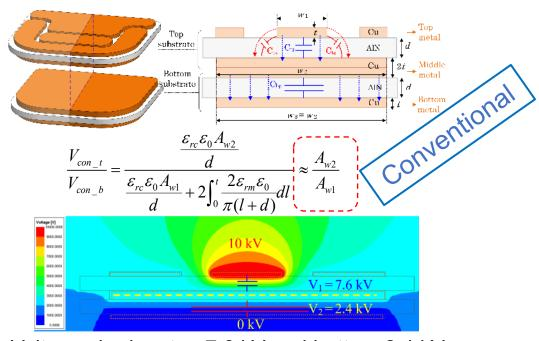
Voltage sharing: top 7.6 kV and bottom 2.4 kV
