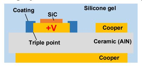
Nano particles added to the coating layer
