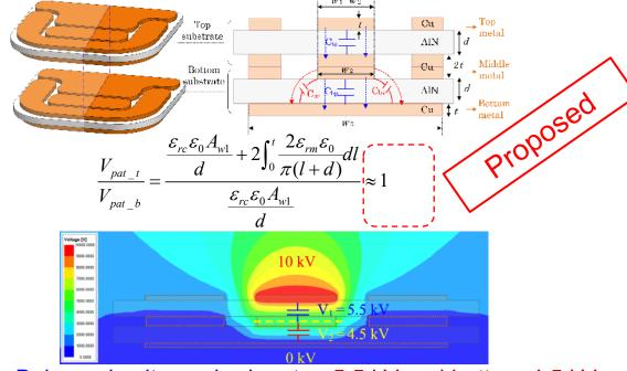
Balanced voltage sharing: top 5.5 kV and bottom 4.5 kV.
