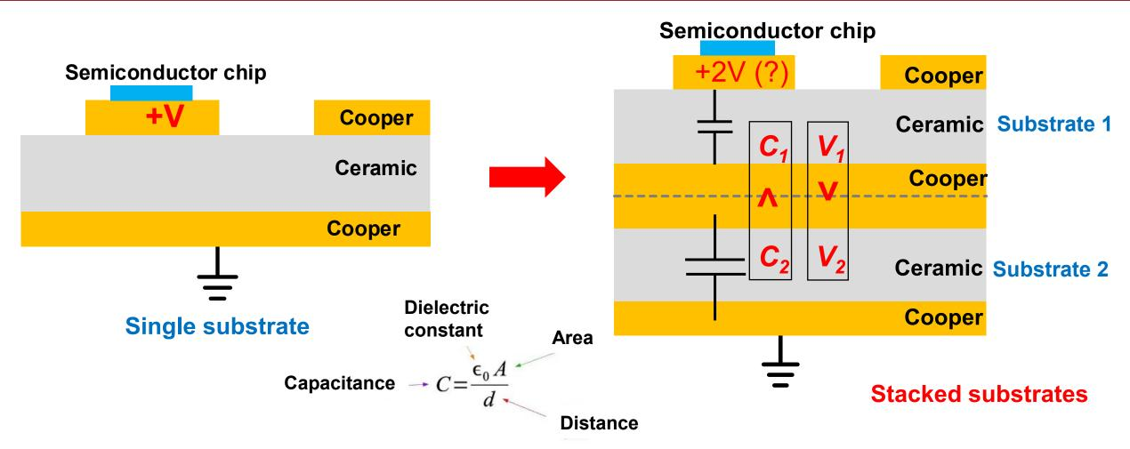
Directly stacking of substrates fails to reduce electric field due to unbalanced voltage sharing.
