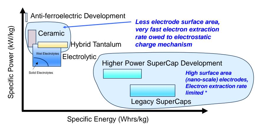
Specific Energy = (V x I x t)/mass Specific Power = (V x I)/mass \* Think of moving embedded electrons out of small pockets
