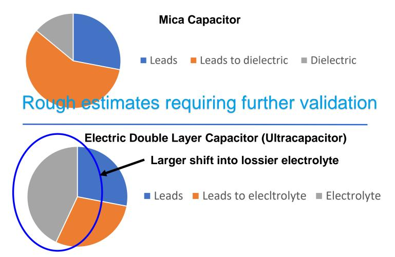
Larger % heating in electrolyte shifts utility away from adopting Electric Double Layer Capacitors in WBG-based high ripple filtering applications
