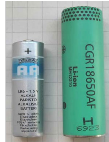
18650 cell format used in 85 kWh Tesla battery
