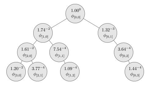
Figure 3.3: Tree structure of the coefficients of a two dimensional PCE with a total-degree basis of order 3. For clarity we only depict one connection per node, but in d dimensions a node of a given degree p will be a child of up to d nodes of degree p-1. For example, not only is the basis  $\phi_{[1,1]}$  a child of  $\phi_{[1,0]}$  (as depicted) but it is also a child of  $\phi_{[0,1]}$
