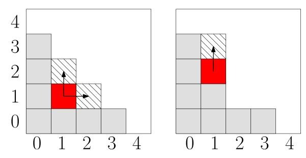
Figure 3.5: Identification of the admissible indices of an index (red). The indices of the current basis  $\Lambda$  are gray and admissible indices are striped. A index is admissible only if its backwards neighbors exists in every dimension.
