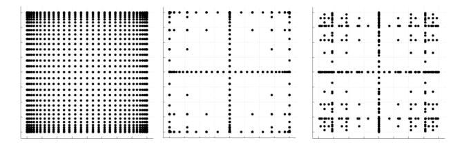
Figure 3.1: Two-dimensional grid comparison with a tensor product grid using Clenshaw-Curtis points (left) and sparse grids  $\mathcal{A}(5,2)$  utilizing Clenshaw-Curtis (middle) and Gauss-Legendre (right) points with nonlinear growth.
