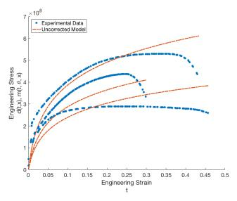
Figure 5.7: Graphs of the calibration data d(t,x) and uncorrected calibrated model  $m(t, \theta, x)$  for configurations (temperatures) x = 373.15K, x = 673.15K, and x = 973.15K.
