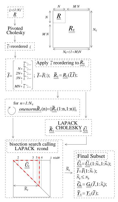
Figure 6.1: A diagram with pseudo code for the pivoted Cholesky algorithm used to select the subset of equations to retain when  $\underline{\underline{R}_{\nabla}}$  is ill-conditioned. Although it is part of the algorithm, the equilibration of  $\underline{\underline{R}_{\nabla}}$  is not shown in this figure. The pseudo code uses MATLAB notation.
