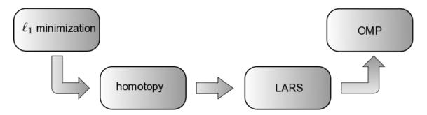
Figure 3.2: Bridging provably convergent  $\ell_1$  minimization algorithms and greedy algorithms such as OMP. (1) Homotopy provably solves  $\ell_1$  minimization problems [44]. (2) LARS is obtained from homotopy by removing the sign constraint check. (3) OMP and LARS are similar in structure, the only difference being that OMP solves a least-squares problem at each iteration, whereas LARS solves a linearly penalized least-squares problem. Figure and caption based upon Figure 1 in [39].
