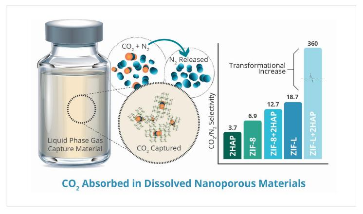
Process for achieving high CO<sub>2</sub>/N<sub>2</sub> selectivity through liquid phase gas capture.
