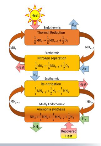
The STAP process consists of two cycles. The first cycle (top) illustrates nitrogen separation from air using concentrated solar heat. The second cycle (bottom) ammonia production at pressure an order of magnitude lower than HB.
