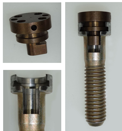
The tamper-resistant fastener consists of a specialized cap and bolt (at right). The bolt (lower left) is laterally slotted and includes a cap retaining area. The cap (upper left) features a square, foot-like section at its base that applies torsion when rotated.
