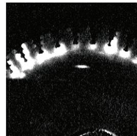
*Above: An infrared camera and an ultrasonic horn (21 kHz) inspects a coated engine part. At left, the resulting thermal image show areas of dynamic thermal strain within the engine part.*
