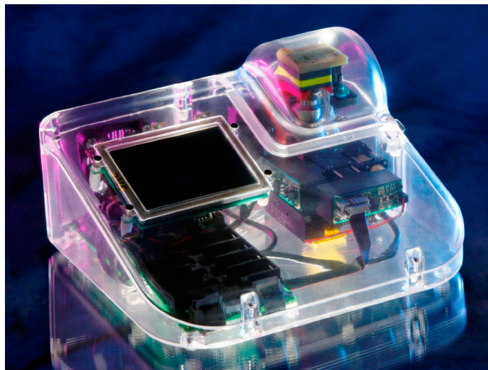
Sandia's RapiD x can analyze drops of blood or saliva in a doctor's office, enabling low-cost, rapid diagnoses during an office visit.
