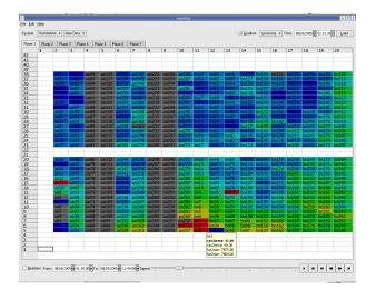
Figure 3. OVIS display of a set of racks of our Thunderbird cluster. Racks 11-20 are the 10 racks on the right side of the figure.
