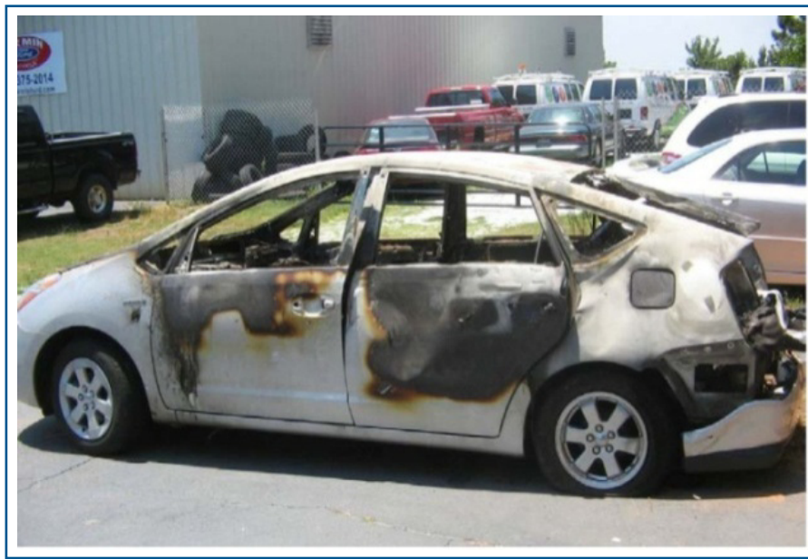
FIG. 2. Full vehicle loss from battery pack thermal runaway in an aftermarket modified vehicle.
