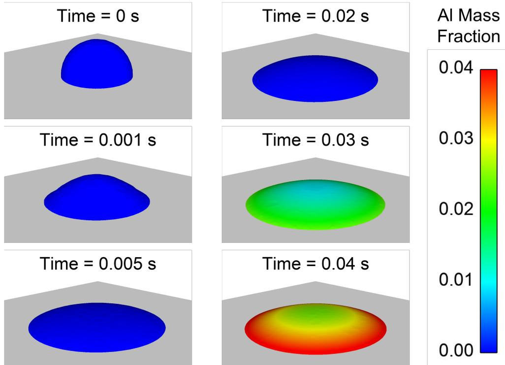
Figure 6: Depiction of FEM sessile drop shapes at different simulation times. The drop coloring corresponds to the aluminum mass fraction as indicated by the colorbar on the right.
