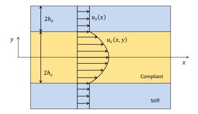
Figure 2. Axial displacement fields in the composite layers.
