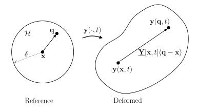
Figure 1. The deformation state  $\underline{\mathbf{Y}}$  maps a bond  $\mathbf{q} - \mathbf{x}$  into its deformed image.
