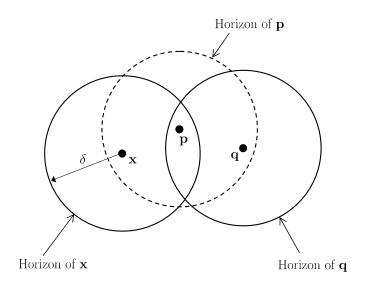
Figure 2. Point  $\mathbf{q}$  interacts indirectly with  $\mathbf{x}$  even though they are outside each other's horizon because they are both within the horizon of intermediate points such as  $\mathbf{p}$ .
