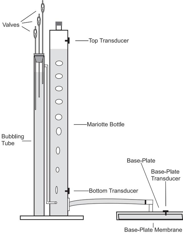
**Figure 1.** Schematic of the tension infiltrometer. The base plate (on the right) is in contact with the sampled medium. Transducers are used to determine the flux rate from the device and the applied tension at the base plate.
