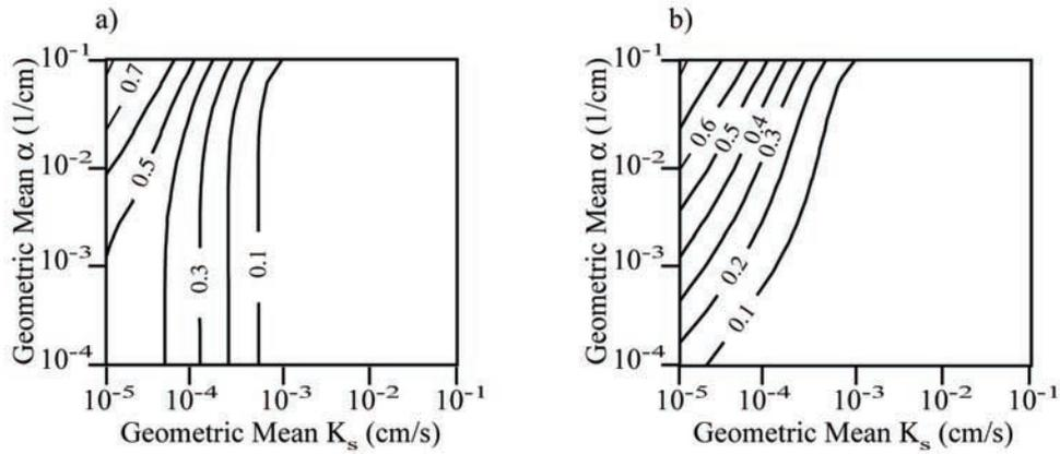
**Figure 2.** Fraction of points discarded as a function of parameter space with (a) observation error and (b) also with contact error.
