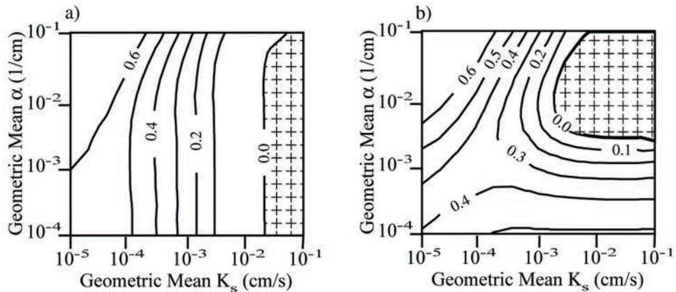
**Figure 7.** Correlation coefficients for  $\ln(\hat{\alpha})$  and  $\ln(\hat{K}_s)$  as a function of parameter space: (a) with measurement error only and (b) also with contact error. Regions with correlation coefficients equal to zero are patterned.
