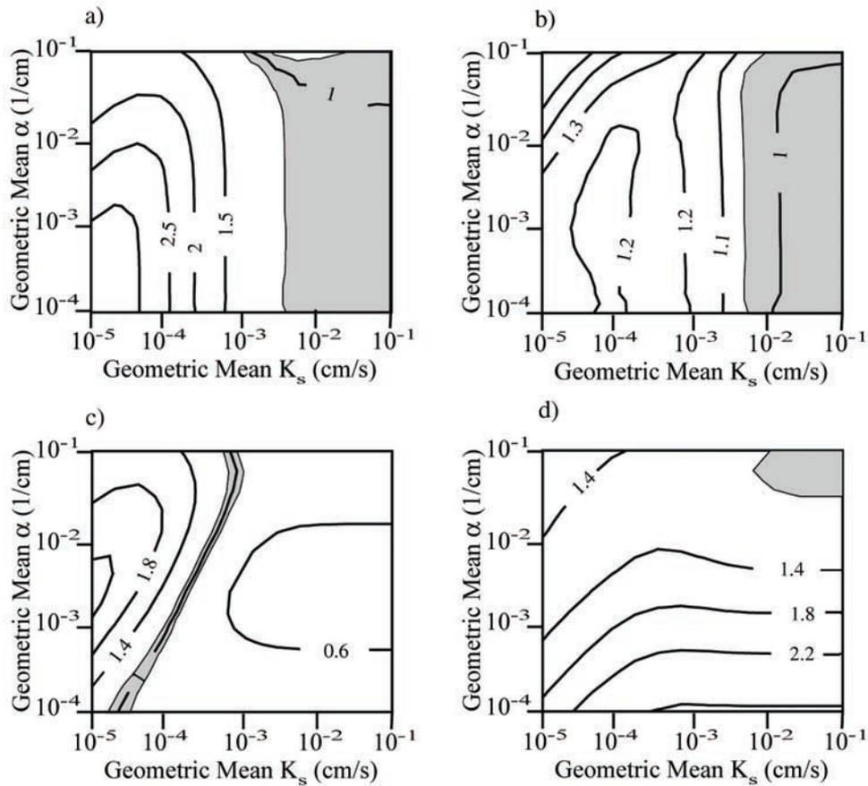
**Figure 4.** Bias in the variance of (a)  $\ln(\hat{\alpha})$  and (b)  $\ln(\hat{K}_s)$  estimated with observation errors alone and bias in the variance of (c)  $\ln(\hat{\alpha})$  and (d)  $\ln(\hat{K}_s)$  estimated with both observation and contact errors.
