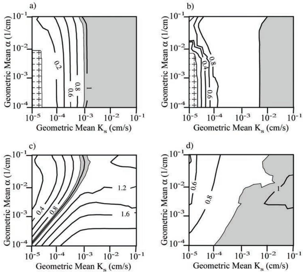
**Figure 6.** Bias ratio for variogram model parameters of  $\ln(\hat{K}_s)$ : (a) model variance with measurement errors only, (b) correlation length with measurement error only, (c) model variance with contact error, and (d) correlation length with contact error.
