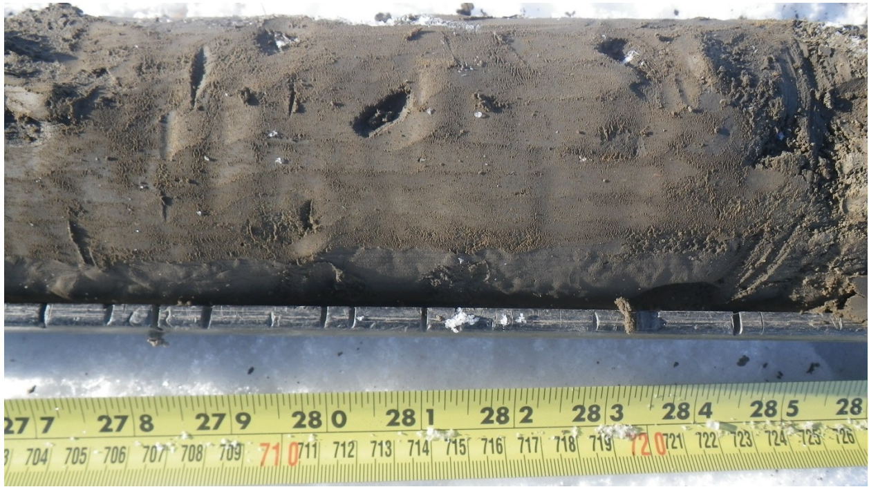
Figure B-6. Borehole PM-1-1, unfrozen silty clayey very fine sand, 705-725 cm.
