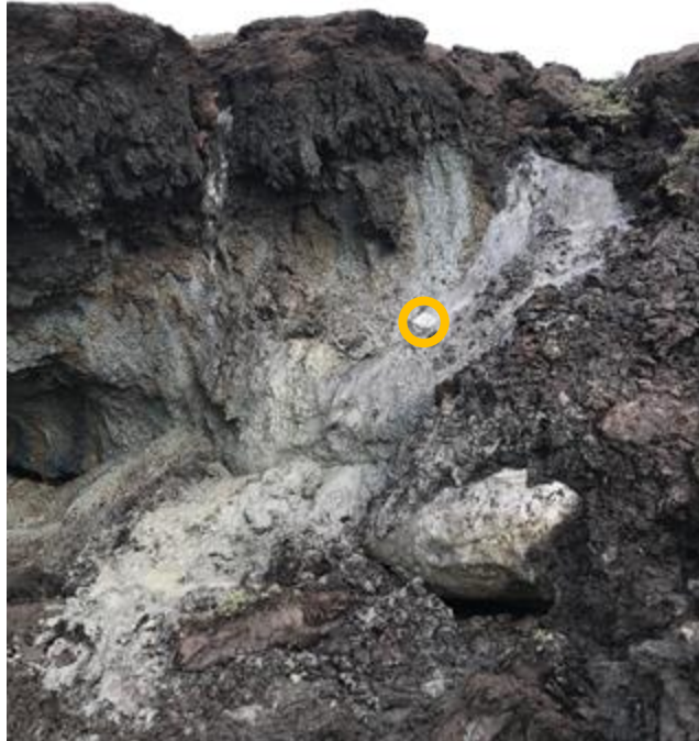
Figure 2.2-2. Field photo showing the installation of the 4-channel data logger (inside gold circle) and thermistor strings in the bluff face at Drew Point.
