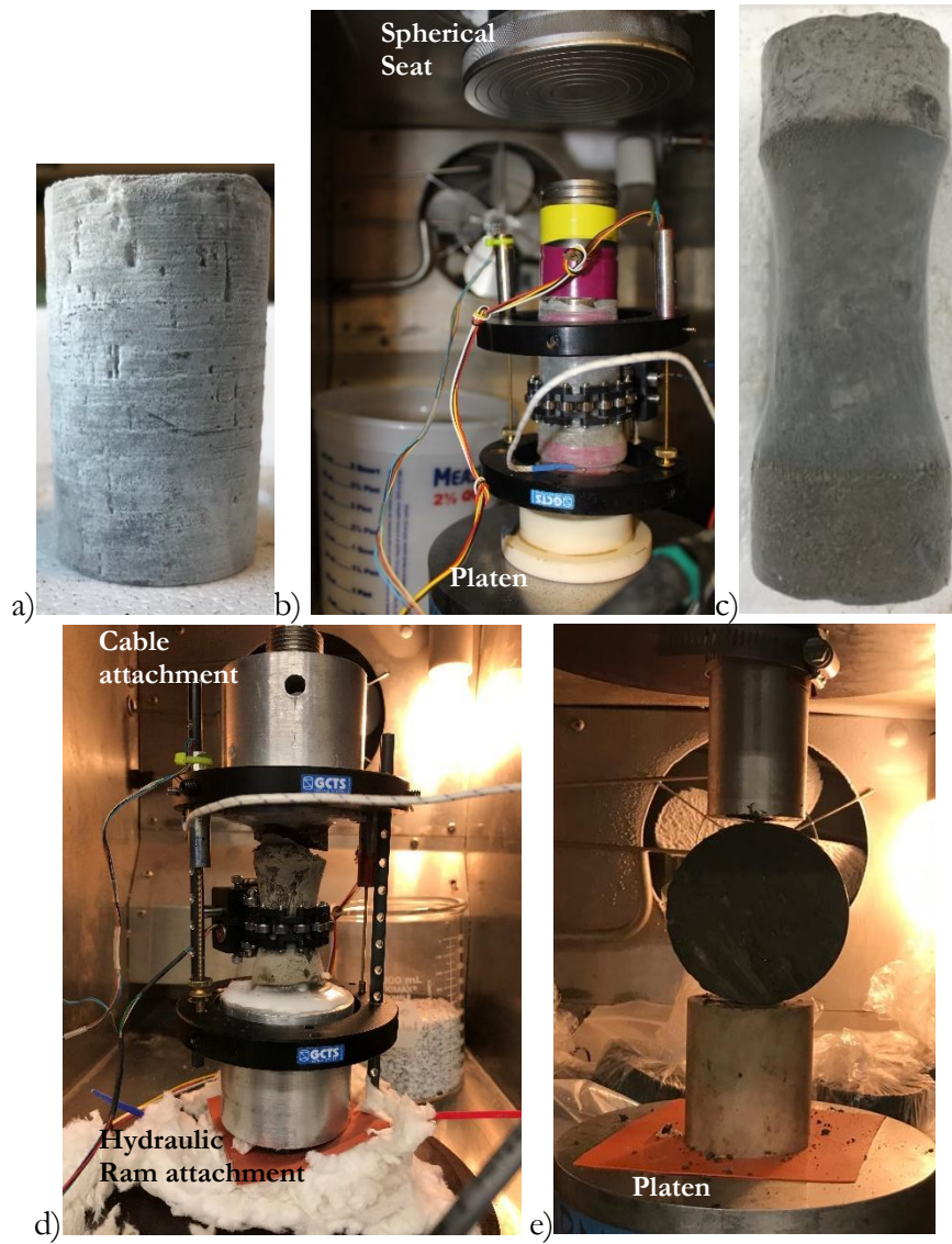
Figure 3.5-1. Experimental setup for the different types of testing. a) Prepared UCS geometry on sample PM1-1 303-310. b) Deformed UCS experiment on sample PM 1-1 303-310. c) Prepared DT geometry on sample PM1-3 512-522. d) Deformed DT experiment on sample PM1-1 213-232.5. e) BTS experiment on DP 1-1 356-371.
