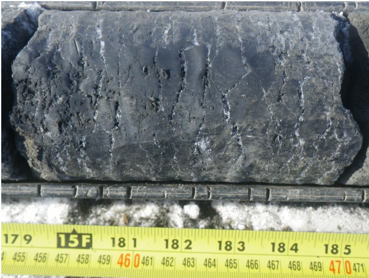
Figure B-4. Borehole DP-1-1, silty clay, braided to reticulate cryostructure, 455-470 cm.
