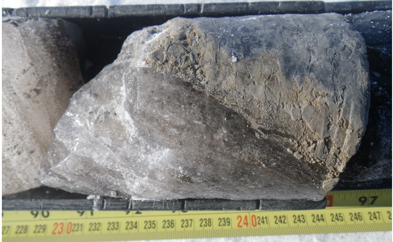
Figure B-12. Borehole DP-2'-2, ice wedge / silty clay boundary, 230-245 cm.
