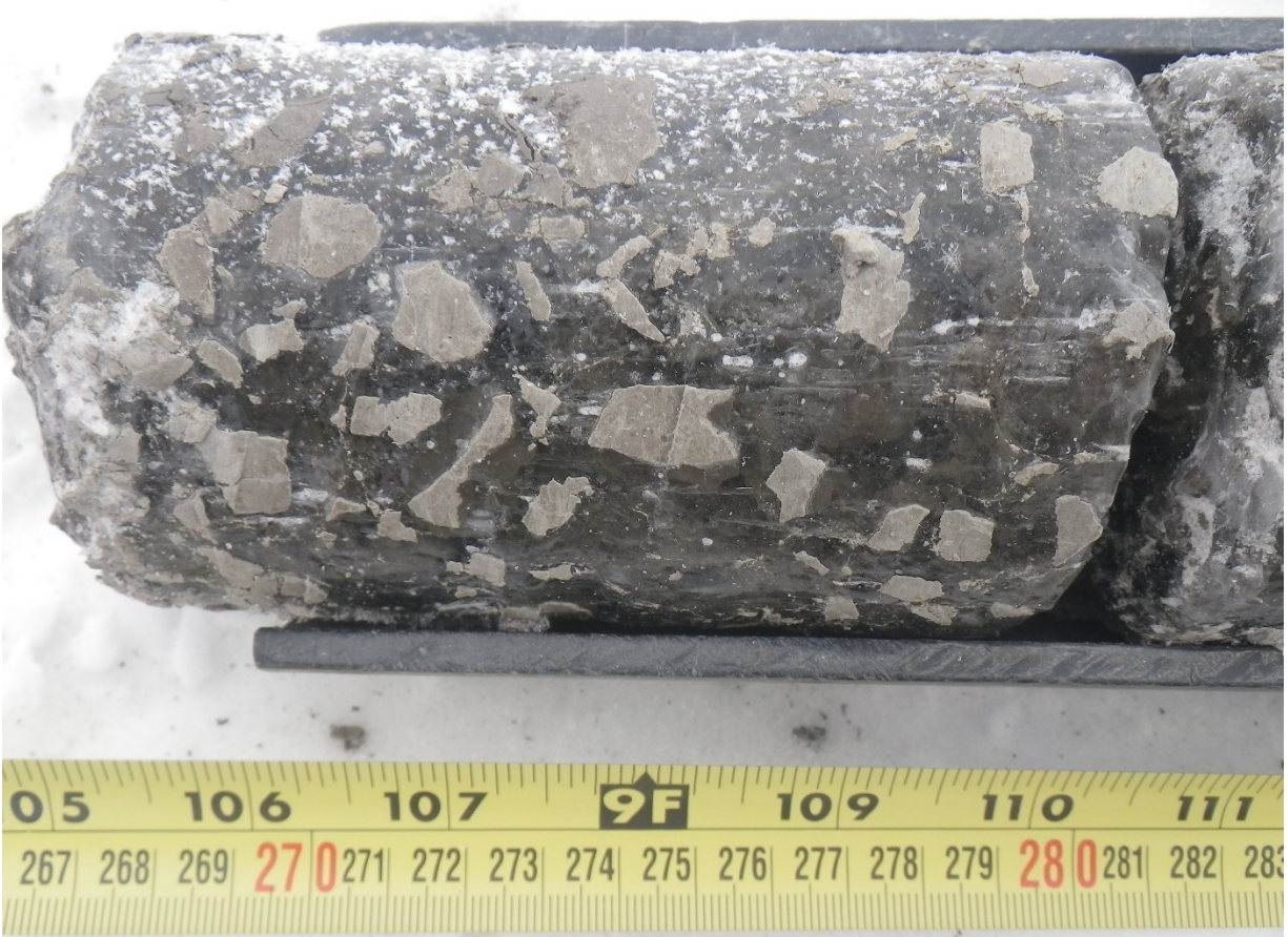
Figure B-14. Borehole DP-1-2, ice-rich silt with ataxitic cryostructure, 265-280 cm.
