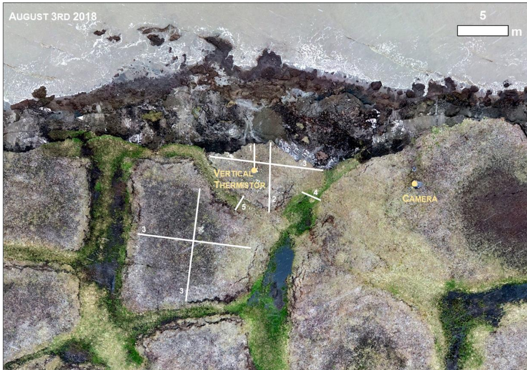
Figure 5.3-1. Image of vertical thermistor location with dimensions overlaid of the polygon size and ice wedge width on August 3 rd 2018. The following dimensions correspond with the lines identified in the plot: 1. 2.62m, 2. 6.5m, 3. 10.8m, 4. 5.65m, and 5. 3.0m.
