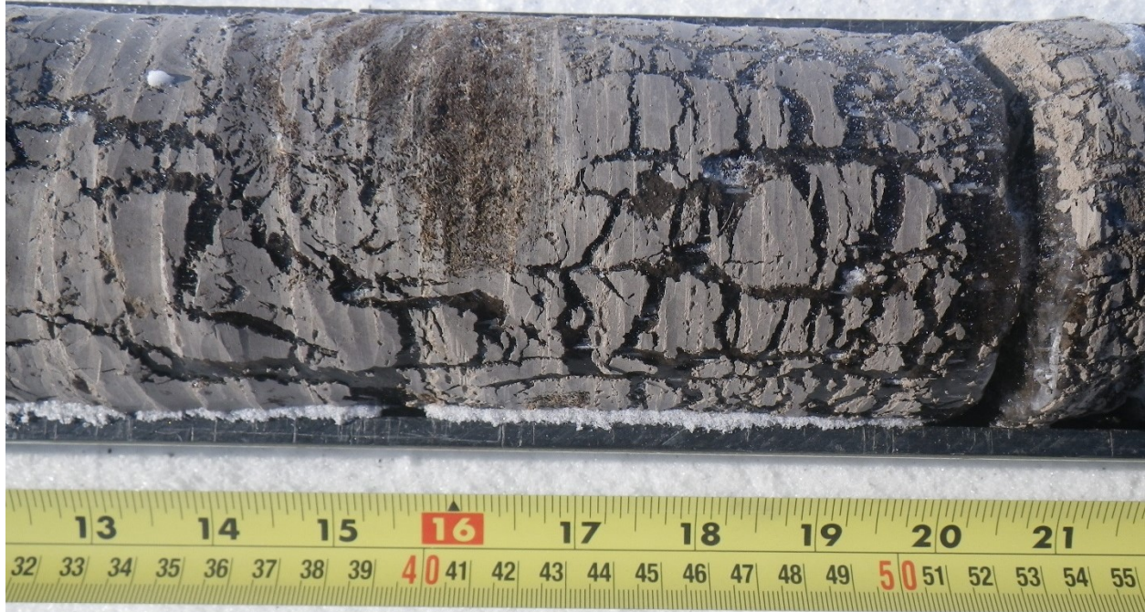
Figure B-10. Borehole DP-2'-2, silt with reticulate cryostructure, 30-55 cm.
