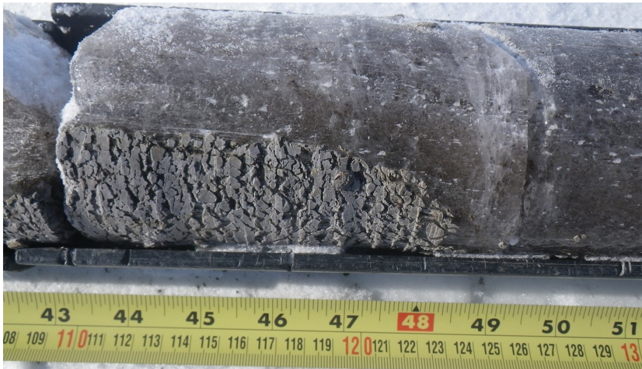
Figure B-11. Borehole DP-2'-2, ice wedge / silt boundary, 110-130 cm.
