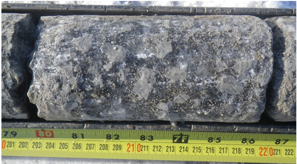
Figure B-3. Borehole DP-1-1, ice-rich silt with ataxitic cryostructure, 200-220 cm.
