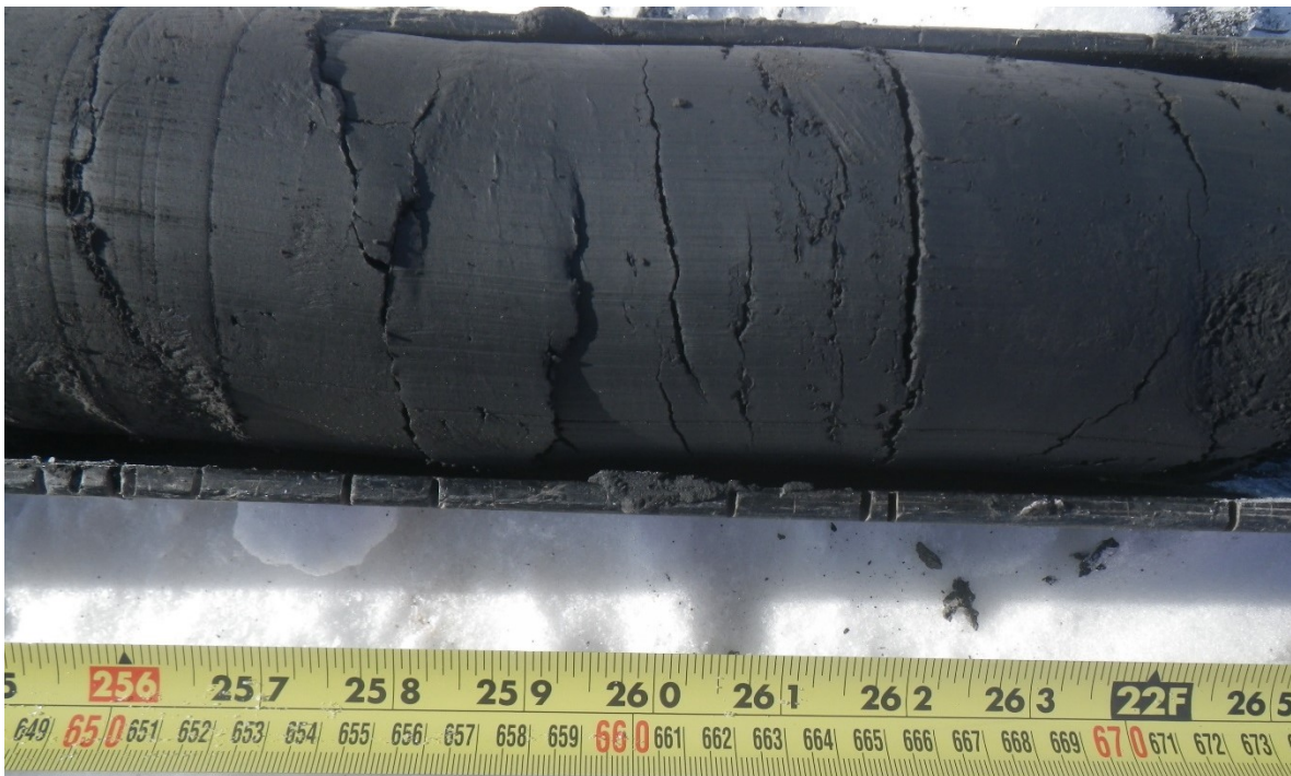
Figure B-9. Borehole DP-1-1, unfrozen silty clay, 650-670 cm.
