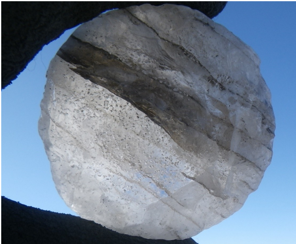
Figure B-7. Borehole PM-1-2, thermokarst-cave ice with vertical frost cracks, ~120-130 cm.
