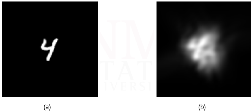
Figure: PSF intensity image of an extended source object: (a) source object (b) intensity image for \frac{D}{r_0} = 10
