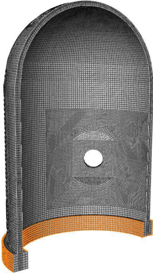
Figure E 6.10 Part of the containment model showing the basemat nodes, which are constrained in the vertical and horizontal directions.
