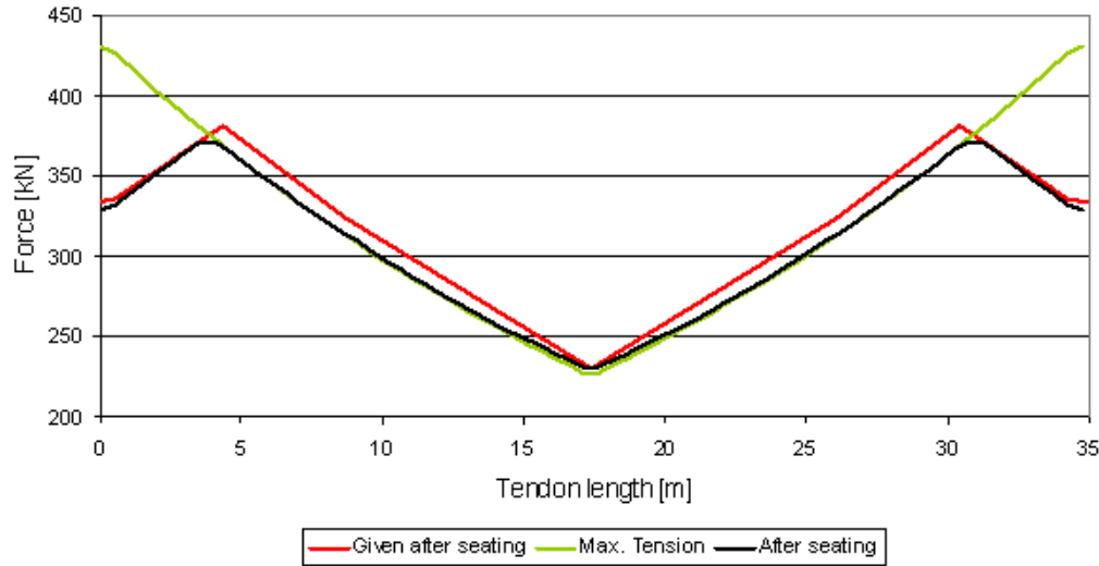
Tendon after prestressing
