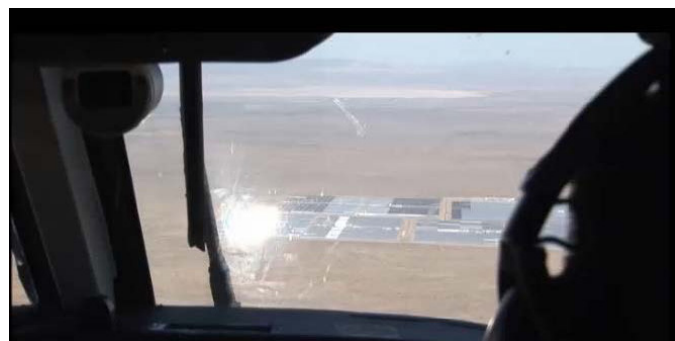
Glare from a large photovoltaic array, observed from C-12 cockpit at Kramer Junction, California (photo from Air Force Flight Test Center 412 TW at Edwards AFB, approval #13166).
