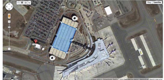
Screen image of SGHAT analysis of Manchester/Boston Regional Airport. PV array (blue outline) and observation points (red marker) are entered using tools integrated with Google Maps.
