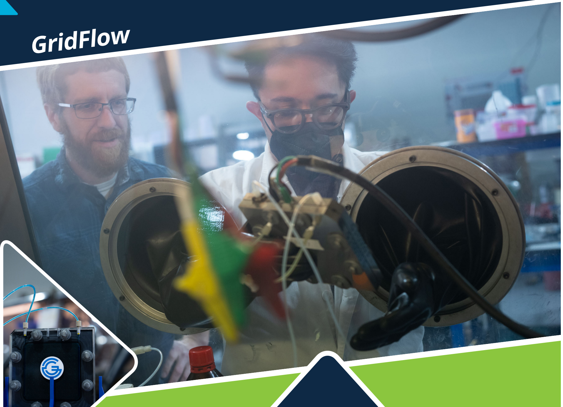
Above: Sandia Materials Scientist Leo Small looks on as GridFlow Senior Lab Technician Rudy Parra works on a prototype flow battery inside a glovebox at GridFlow.
