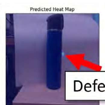
The MAADS system identifies a slight defect to a thermos that would be very difficult to see without machine-learning help.
