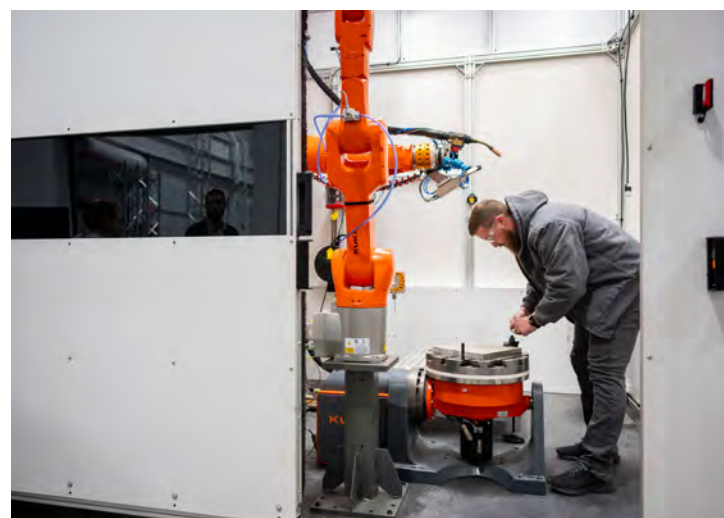
A technologist installs a new base plate on a system for additive manufacturing at CAMINO.
