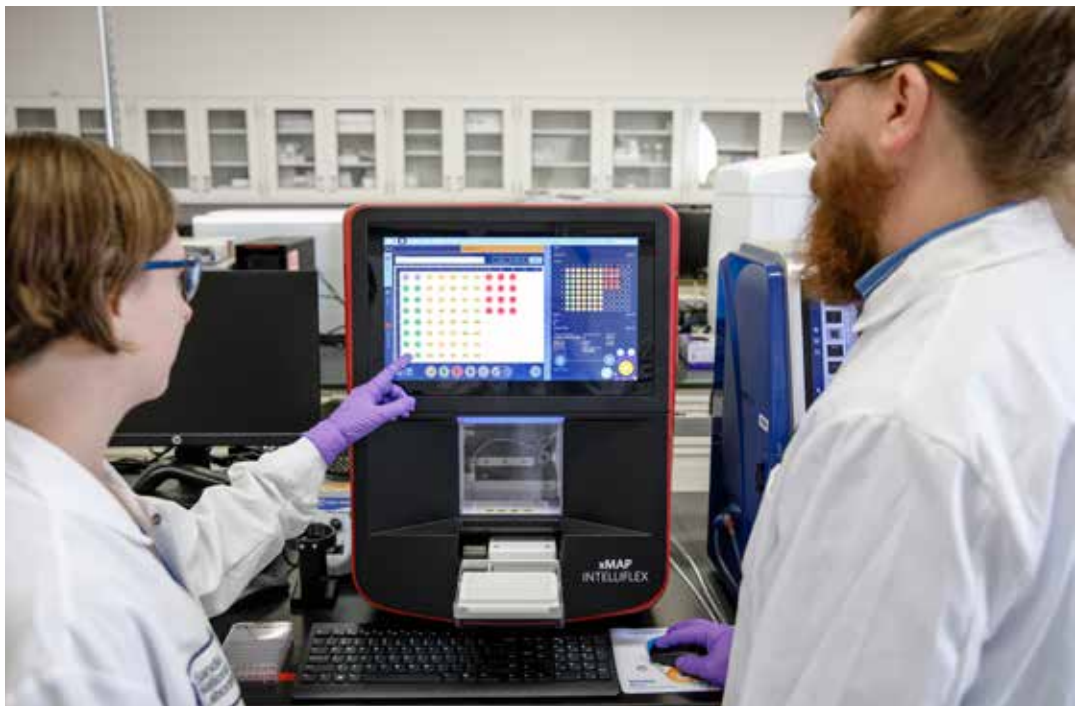
Right: Sandia Researchers Iris Jones and Dylan Johnson leverage the xMAP Intelliflex System to perform high-throughput analysis of protein and gene expression assays for CAPSIID.
