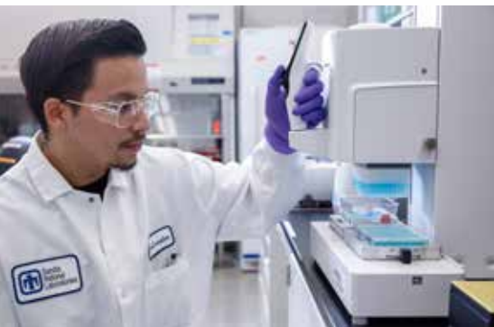
Above: Sandia Technologist Salvador Martinez uses an Integra Viaflow 386 to prepare microtiter plates for high-throughput assays.
