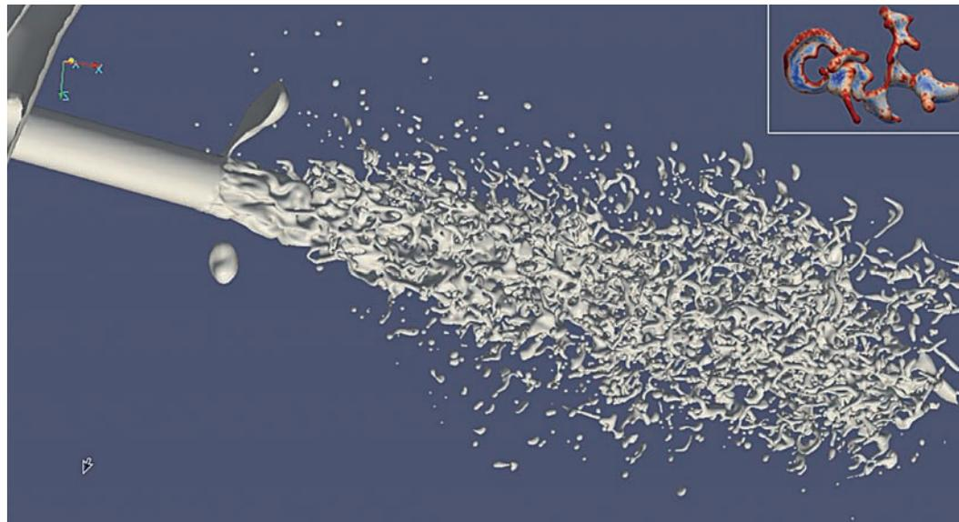
device at the level of accuracy displayed in the figure is limited to a small volume around the injector and requires several weeks of computer time, on a machine such as Red Sky, to collect sufficient spray statistics.
